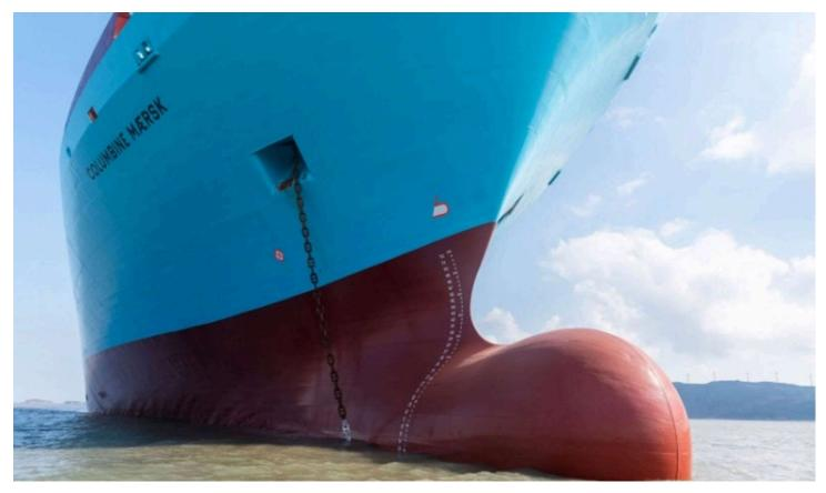
Making changes to a ship's bulbous bow reduces drag and cuts fuel consumption. Photo credit:
